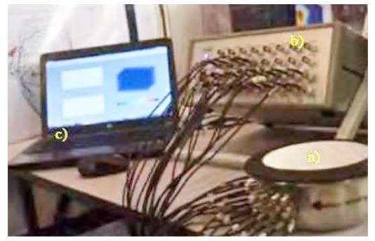
The Schematic System of ECVT : a) Sensor, b) DAS, c) PC.
